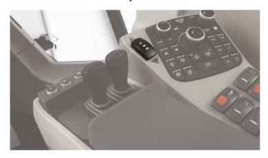
The **TIPSHIFT** function provides operator ease of operation. It is possible to change the direction quickly by pressing a single key without using the gear lever when the machine is moving forward or backward while taking under the load or unloading. This increases productivity and ensures safe operation without the loss of steering control.
