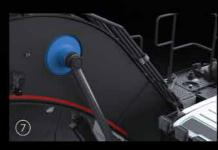
Reinforced boom cylinder cast bearing
