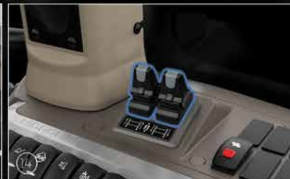
Automatic Control of Stabilizers (**)
