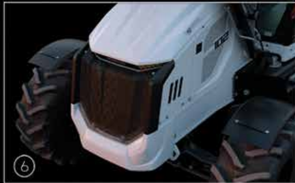
⑥ Durable engine front grille and protection bumper
