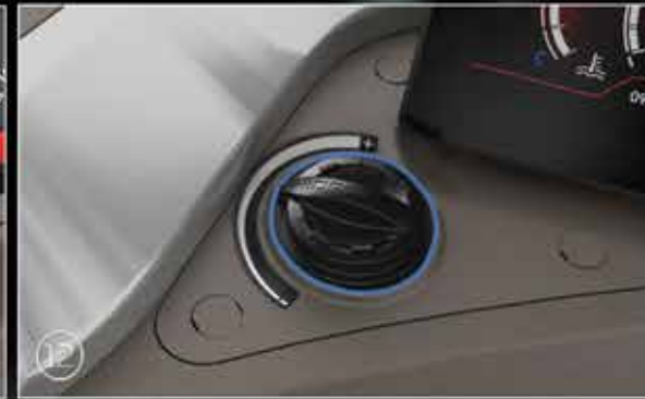
Hand Throttle with Electronic Rotary Control (*)
