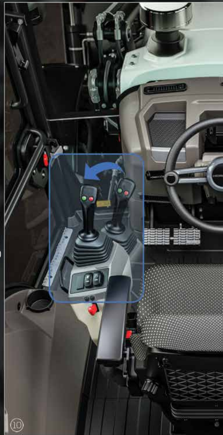
Tilting of the left joystick to some extent for the operator to work more comfortably on the loader side
