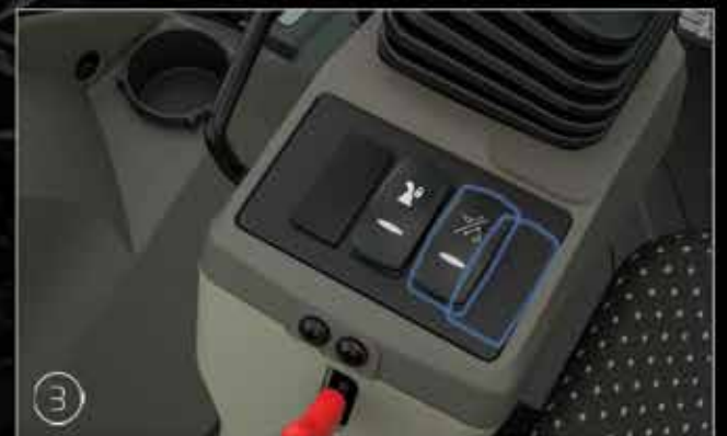
3 Shifter Button for Backhoe or Loader Function
