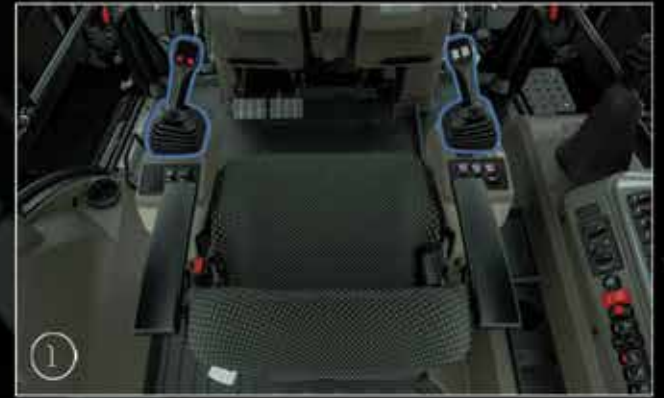
1 Shifter Button for Backhoe or Loader Function
